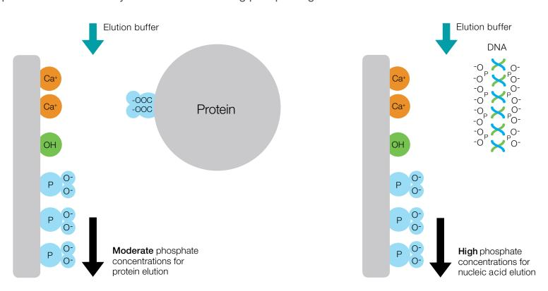
Phosphate gradients are typically used to elute biomolecules bound to CHT by metal affinity interaction. However, NaCl also affects their retention time, indicating a minor contribution by cation exchange.1
