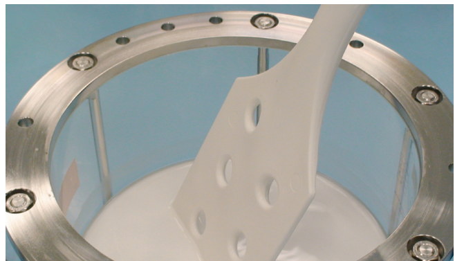
Fig. 4. Use a plastic paddle to manually mix the slurry.
