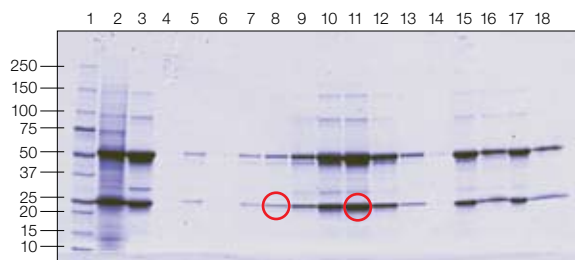
Fig. 3. SDS-PAGE analysis of chromatographic fractions. 1, Precision Plus Protein™ standard; 2, MAb cell culture harvest; 3, protein A capture eluate. Lanes 4–16 show UNOsphere Rapid S media chromatography: 4–5, flowthrough 1 and 2; 6, wash; 7–14, elutions 1–8; 15, pooled elution fractions 3–6; 16, strip. Lanes 17 and 18 show UNOsphere Q media chromatography: 17, flowthrough; 18, strip. The bands circled in red correspond to the bands used for mass spectrometry analysis in Figure 4.
