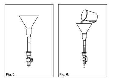
5. Affix a funnel to top of column, close column exit, and add enough buffer to fill 20% of column (Figure 5).
