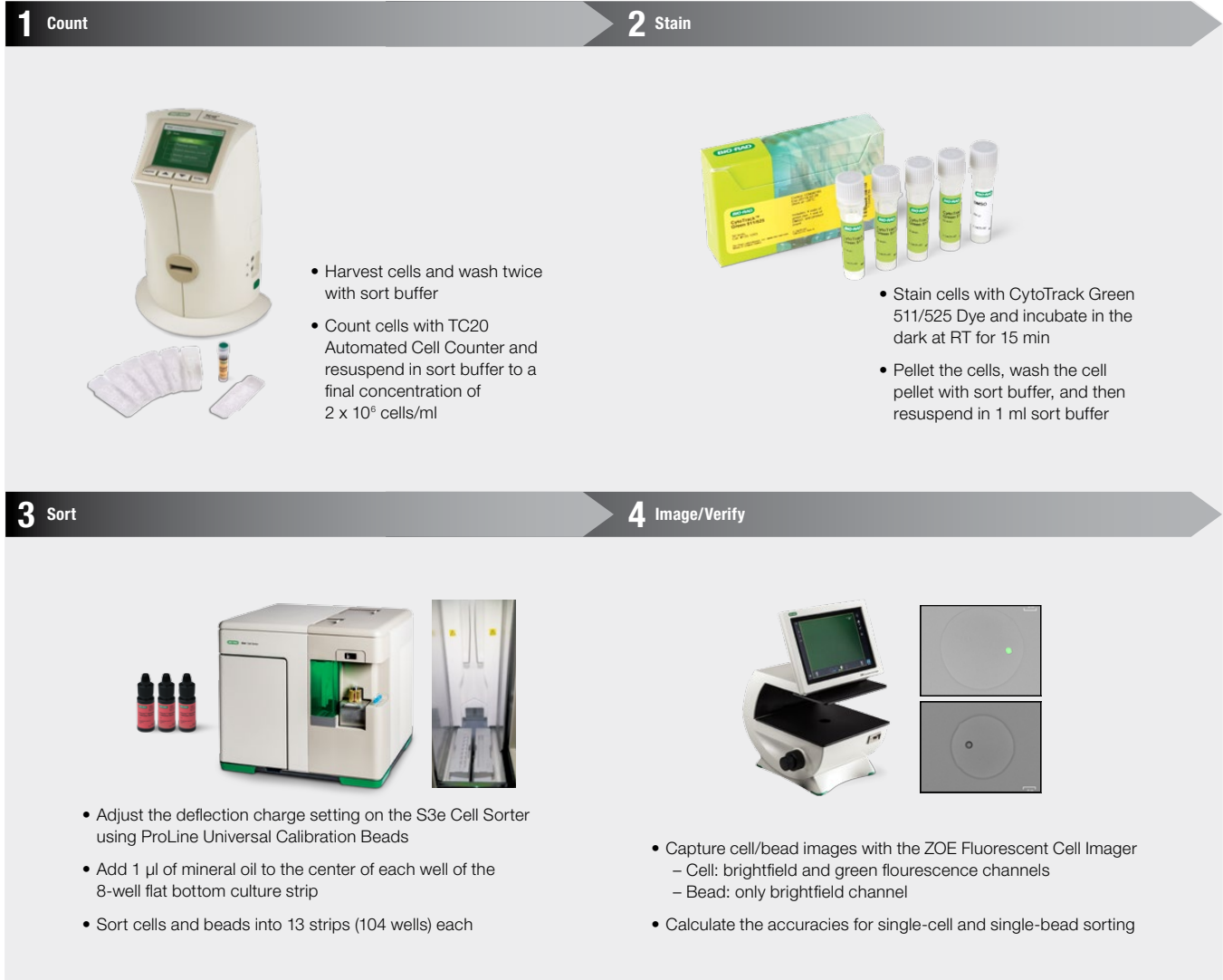
Fig. 3. Single-cell sorting verification workflow. Depiction of a simple workflow to verify the accuracy of single-cell sorting on the S3e Cell Sorter. The ZOE Fluorescent Cell Imager serves as the final QC/verification step.
