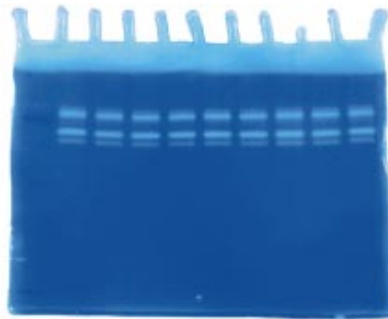
10% Zymogram Ready Gel with Gelatin, 10 well, catalog number 161-1022.
