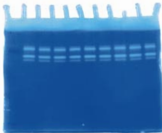
10% Zymogram Ready Gel with Gelatin, 10 well, catalog number 161-1113. Samples: lane 1, blank, lanes 2-10, Collagenase F. Stained with Coomassie Blue R-250.
