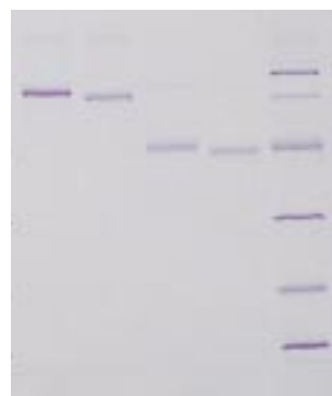
Coomassie stained 12% Ready Gel. Human transferrin and ovalbumin were deglycosylated with the Enzymatic Deglycosylation Kit. Mobility shift indicates proteins were deglycosylated.
