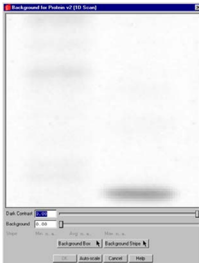
Fig. 3-20. Dark Contrast adjustment reveals true levels of background in the image.
