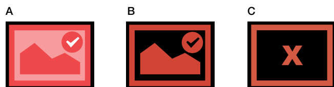
Fig. 15. Color channel icons in Merge mode. A , active: color channel with selected image, the image is displayed; B , inactive: color channel with selected image, the image is hidden; C , empty: color channel for which no image was selected.
