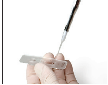
Fig. 9. Loading the counting slide.
