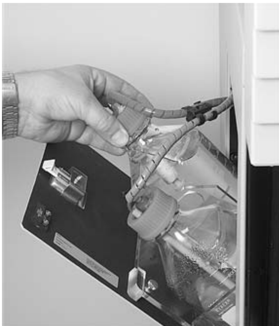
Figure 2-10. DI water and waste bottle installation.
