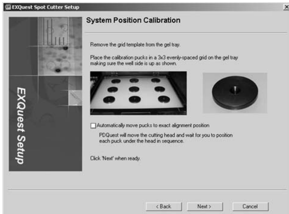
Figure 3-9. System position calibration.
