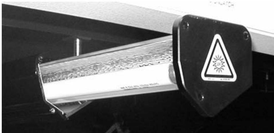
Figure 10-2. UV EPI Lamp Partially Removed
