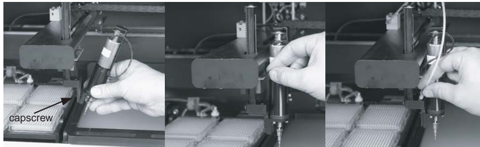
Figure 2-8. Membrane cutting head installation.
