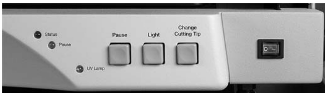
Figure 1-10. Status light and front panel controls.
