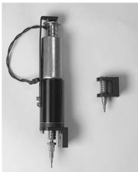
Figure 1-5. EXQuest membrane head (left) (Patent pending) and gel cutting head (right).
