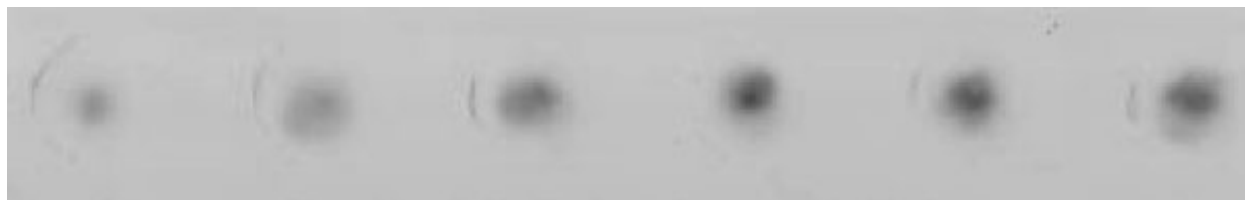
Fig. 25. Representative bombardment showing penetration of 1.6 \mu\text{m} gold particles into Parafilm Laboratory Film at (left to right) 100, 200, 300, 400, 500, and 600 psi using the Helios Gene Gun.
