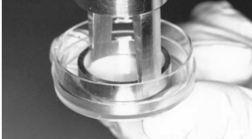
Fig. 18. Correct placement of the Gene Gun when transfecting cells in vitro (photo courtesy of Auragen, Inc.).
