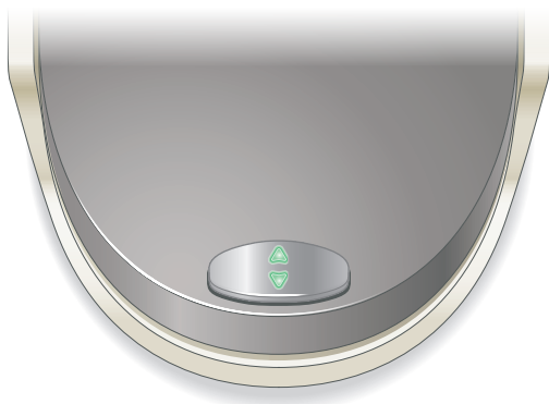
Fig. 3. The power is on when the two arrows on the push button illuminate green.
