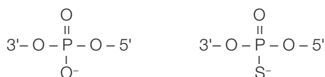
Fig. 1. Chemical structure of phosphodiester (left) and phosphorothioate (right). The replacement of one nonbridging oxygen with sulfur makes the phosphorus center chiral.
