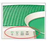
Before you start a run, check the indicator lights to ensure the instrument is ready. For information, see Table 10.
