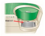
**Important:** Make sure the tabs on the plate holder are securely clamped and the plate lays flat. Otherwise, the sampling needle can strike the lid and damage the instrument.
